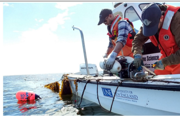
Figure 2. Authors installing load cells in mooring line to measure tensions during wave and current forcing
