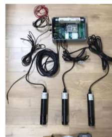
Fig.2 Layout of the wireless sensing embedded system
