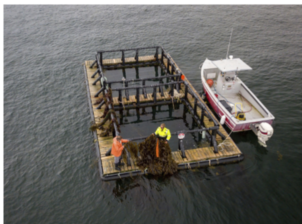
Figure 1. Prototype integrated multi-trophic aquaculture raft developed by the University of New Hampshire to culture, steelhead trout, blue mussels and sugar kelp.
