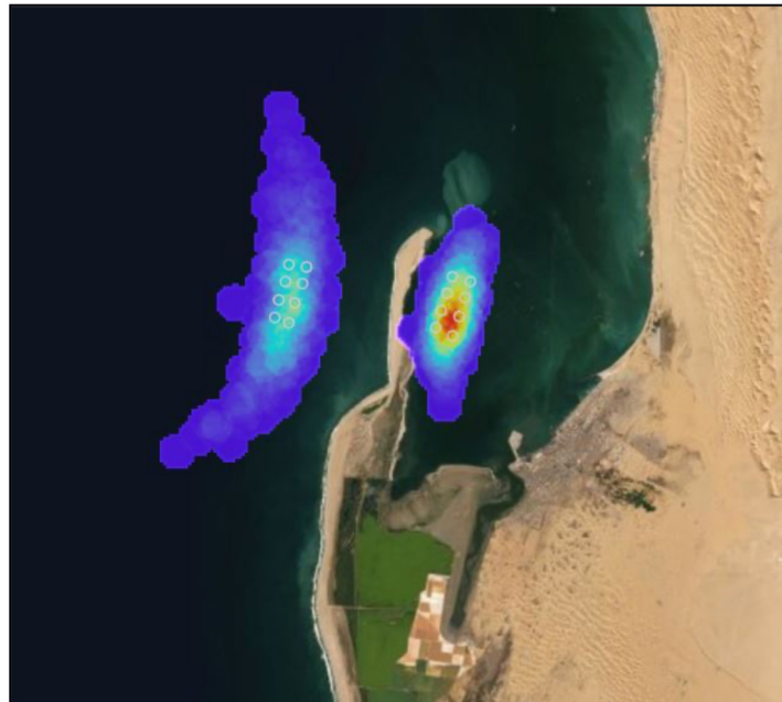
Figure 1: The effect of stronger currents on the grid outside the bay can be seen through the results of a deposition model. The grid on the left has a large area of effect but lower area of significant impact (area in red).
