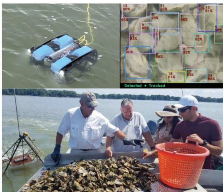
Figure 1. (A) Underwater remotely operated vehicle (ROV) platform. (B) Computer vision identification and assessment of on-bottom oysters. (C) Oyster dredging operation on the Chesapeake Bay in Maryland.
