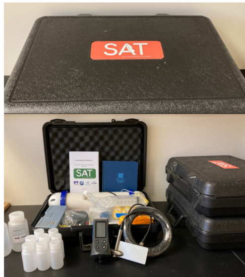
Figure 1. Site Assessment Toolkit (SAT ® ) designed, assembled, and tested in Alaska for kelp mariculture.
