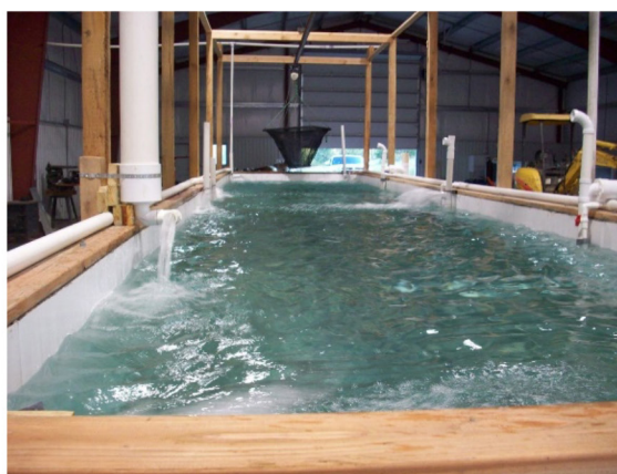
Figure 1; Concreted-filled, prefabricated PVC forms holding 4,000 gallons within climate-controlled, zero-discharge, RAS prototype at a private farm in Missouri.
