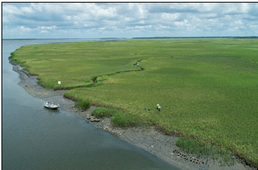
Figure 1. Photograph from Big Bay Creek, a tributary of the South Edisto River, taken on August 19, 2021. The photograph includes a number of living shoreline materials installed on June 1, 2016. Over the course of 5 years there has been expansion of salt marsh habitat seaward from the naturally-occurring marsh edge for all treatments except the negative control (fourth experimental plot from left to right).
