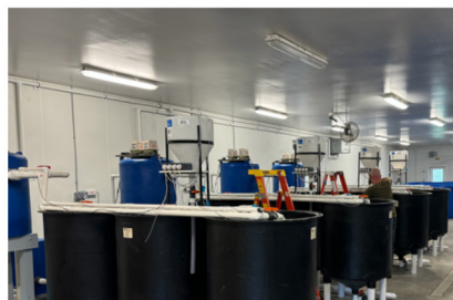
Left: Replicated RAS with 12 tanks, feeders and unit operations. Right: Skimmer to enhance surface properties for larval swim bladder inflation. (Photos: Hall, Frinsko)
