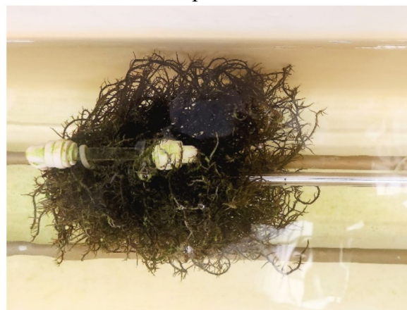
Fig 1: Biomass panel with pitot tube.
