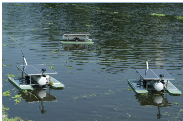
Figure 1: This fleet of dual paddlewheel autonomous surface vehicles may also be in communication with aerial vehicles and should enhance human decision making and management.
