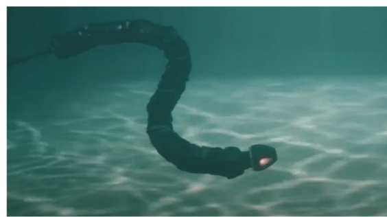
Figure 2: The Mamba, a bioinspired underwater snake robot while swimming.
