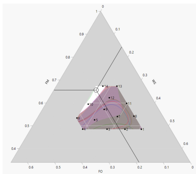
Figure 1. Analysis of the diet response surface at the end of the 20-week feed study. The predicted optimal diet surface area, in white, with the suboptimal regions shaded in. The point is the 90% optimal response with the ratio of 0.6559 fishmeal, 0.1884 fish oil, and 0.1556 wheat starch.
