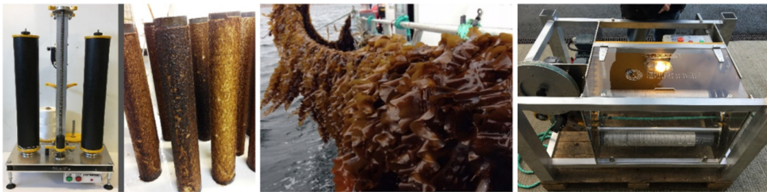
Figure 1: Machines for spinning of seedling strings (left and right), and test result (middle)
