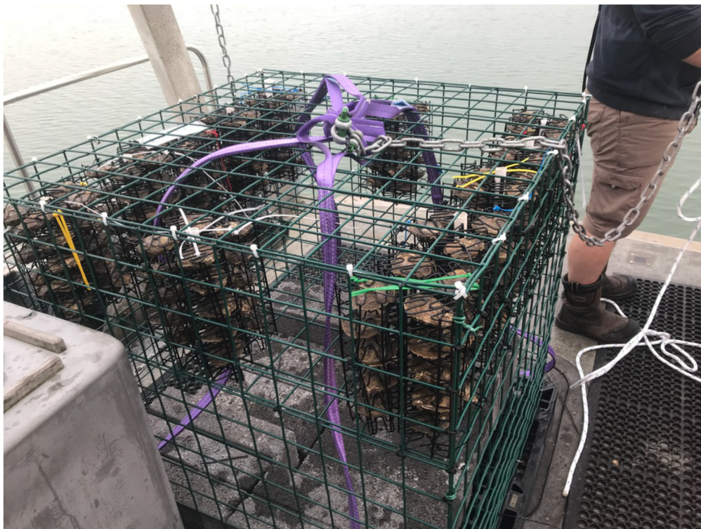
Figure 1. One 1 m 3 gabion to be placed on the seabed. This gabion holds a density of 240 oysters, elevated to a height of 0.8 m from the seabed.
