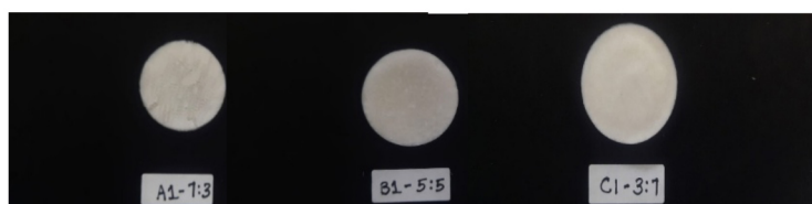
Figure 1. Gelatin Ulvan Scaffolds prepared at different ratios of gelatin & Ulvan
